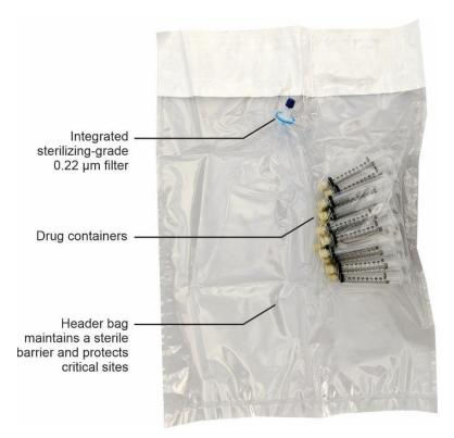
then capping each container. Once the containers are filled and capped, the package is opened, and the sterile-filled containers may be removed.
